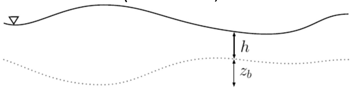
$$W_h : \frac{\partial h}{\partial t} + \frac{\partial(hu)}{\partial x} + \frac{\partial(hv)}{\partial y} = i_h$$
